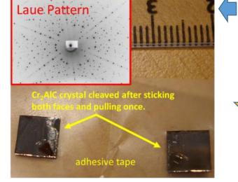
« Big » crystals cannot be mechanically exfoliated down to very thin layers (roughness increases too much after a few exfoliation steps).
