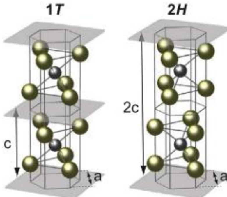
**Figure 3.** Schematic crystal structure of the 1T (left) and the 2H (right) polytype of layered transition-metal dichalcogenides. In the 1T structure, the transition-metal atoms are octahedrally coordinated by chalcogen atoms and the thickness of the repeat unit in the  $c$  direction is one sandwich. In the 2H structure, the coordination is trigonal prismatic and the unit cell is two sandwiches thick.
